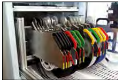
MSD cabinet with feeder rack and SMD Reel rack ESD coated with reel support
