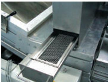
Beyond this, the machine may be equipped with a controlled and integrated exhaust 4-stage filtering system. In addition, a process gas cleaning unit is available optionally.
