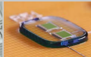
Dam and Fill
