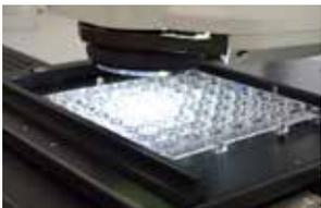
Common to both Lynx EVO and EVO Cam systems it allows a rotating oblique view of 34° from 360° around a feature as well as the expected direct view. Making it easy to see side details around features as well as the usual top surface. Especially useful for joints, holes, pillars and threaded forms.
