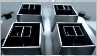
multi-nozzle tool for dip soldering processes
