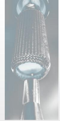
automatic ultrasonic solder nozzle cleaning patented by SEHO
