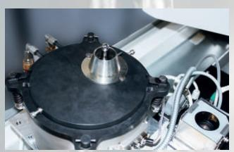
electro-magnetic soldering unit: miniwave or dip soldering processes
