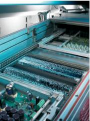
Depending on the assemblies to be processed the various conveyor sections, e.g. in the fluxer, preheating or soldering area, can be set to individual transport speeds. This is of enormous advantage because with many applications the process window will be extended considerably due to this higher machine flexibility.
