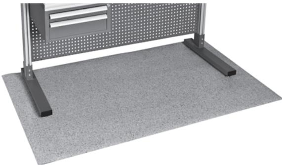
Double-layer anti-static floor mat 2.5 mm thick, abrasion resistant, sound-absorbing, non-flammable, thermally stable, dissipative top layer and conductive bottom layer: dripping time charge from 1000 V to 50 V in less than 0.5 seconds, the resistance of the ground — less than 100 MΩ, the combined resistance — less than 35 MΩ. Various dimensions: 150 mm×200 to 1000×10000 mm.
