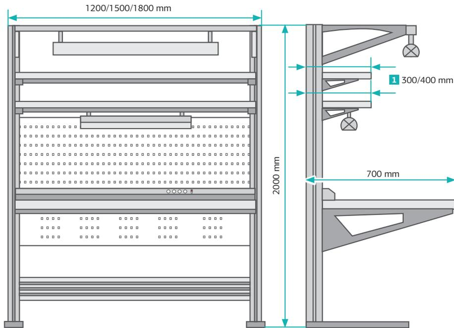
**Alliance automatic** workbenches AL/A are distinguished by elegant design, advanced ergonomics and motorized worktop adjustment system, performed by electric drive and simple control unit. ALLIANCE Automatic allows setting tabletop height easily and quickly by simply pressing a button, which is indispensable in certain working processes.
