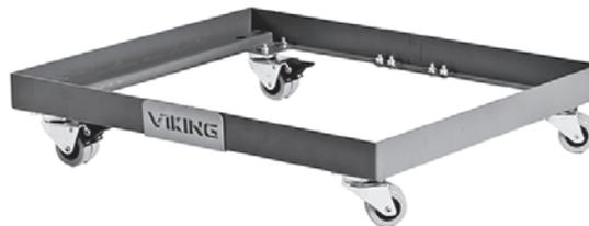
Movable drawer unit support is an additional unit that helps to turn stationary drawer units and cabinets into movable one. It matches all standard cabinets (TMB-01/1 and TMB-02/1) and drawer units (DR-03/1, DR-05/1, DR-07/1 and DR-10/1). Four 50 mm casters, two of which are with brakes.
