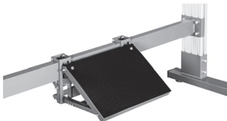
It is only suitable for ALLIANCE series workbenches. The footrest should be mounted to the lower slat and is equipped by a nonskid floor mat. 130° to 160° angle adjustment provides additional convenience for an operator.
