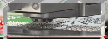
The Paraquda has the ability to be equipped with a wide variety of dispensing valves for solder paste, adhesives or dam & fill materials. Prototypes are easily assembled without the need for stencils, reducing your turnaround time considerably. Expensive stepped stencils can also be eliminated with the dispensing of additional solder paste. It uses the same proven software as the Scorpion, and so delivers identical professional high speed dispensing solutions.
