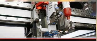
Four processes at the same time. Plug and Play for valve change. Piezo Jet Valve - super high speed for low viscosity. Solder Jet, Volume Displacement, Time/Pressure, Archimedean Screw Valve
