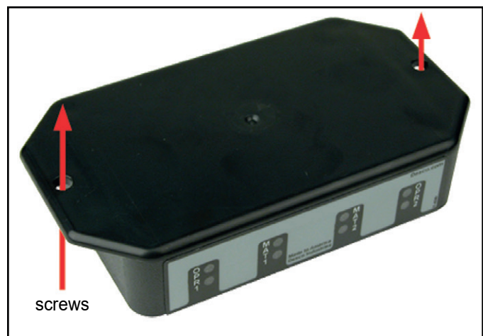
Figure 2. Mounting the Control Unit
