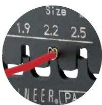
Excellent curling of wire and insulation barrels individually
