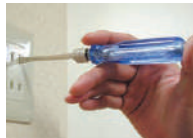
Circuit testing handle (AC80~250V/DC100~300V)
