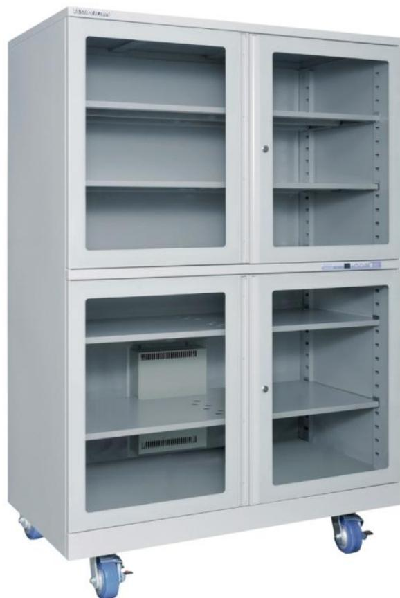
CSD-1104-03 has an outstanding performance for drying moisture sensitive components and PCBs as a result of a high performance drying unit. Humidity can be controlled precisely by digital panel to reach the lowest 3%RH. It is specially designed for moisture sensitive SMD packages to comply with IPC/JEDEC J-STD-033D.
